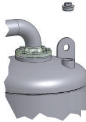
Unscrew the sleeve plug
